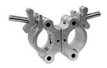
The Swivel Coupler will fasten from 1-1/4" pipe (1.660" OD) to 2.050" OD truss tube. The Swivel-Coupler has wide wing nuts for fastening the clamp
