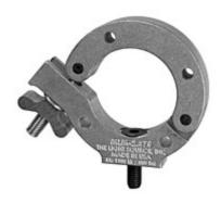
The Monstro-Coupler 2.375 perfectly connects to 2" pipe.(2.375" OD) The Monstro-Coupler 2.375 has a 1/2"- 13tpi countersunk fastener for connecting a fixture. The Monstro-Coupler 2.375 is CNC machined from 6061T-6 aluminum alloy and has a working load limit of 1100 pounds.
