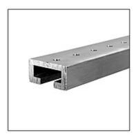
The XYZ Channel and the XYZ Mount make installing LED video walls a breeze. The 6061T6 aluminum alloy channel is pre-drilled on one inch centers for number 12 flathead screws to allow easy mounting to 16" and 24" on center studs. The XYZ mount slides in from the side to any desired location and is locked in place with a set screw. Available in two lengths, 1800 mm and 2400 mm, to match most LED panels.
